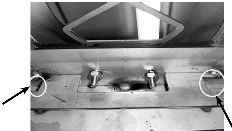
Figure 4: Front mounting slots for Flue Gas Agitator.
