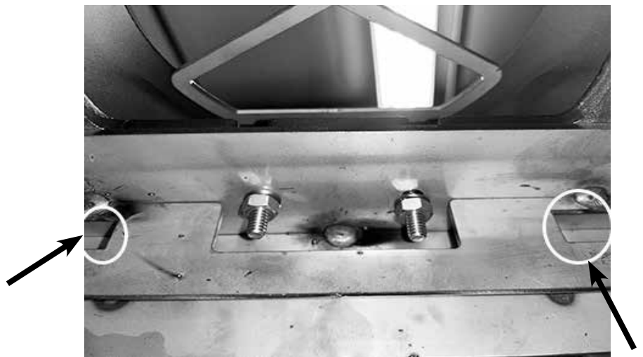
Figure 6: Front mounting slots for Flue Gas Agitator.
