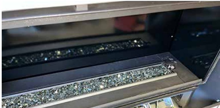
Figure 56: Crushed Glass Media in Burner Tray
