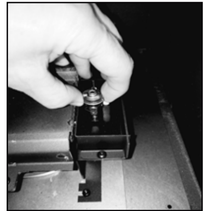
Figure 41: Pilot Head Removal.
