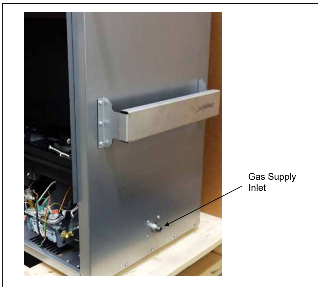
Figure 45: Gas Supply Inlet.
