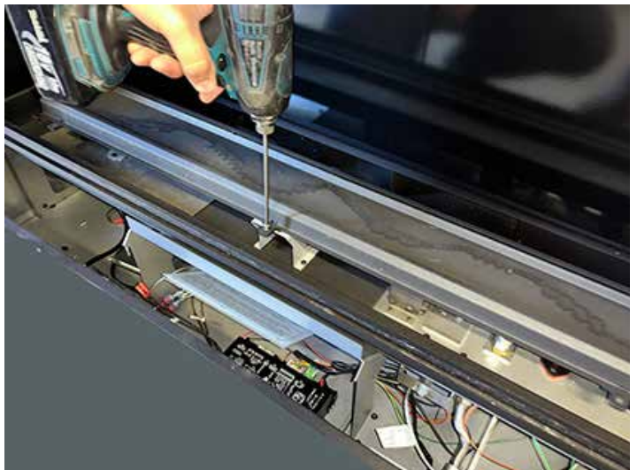
Figure 68: Air Deflector Removal
