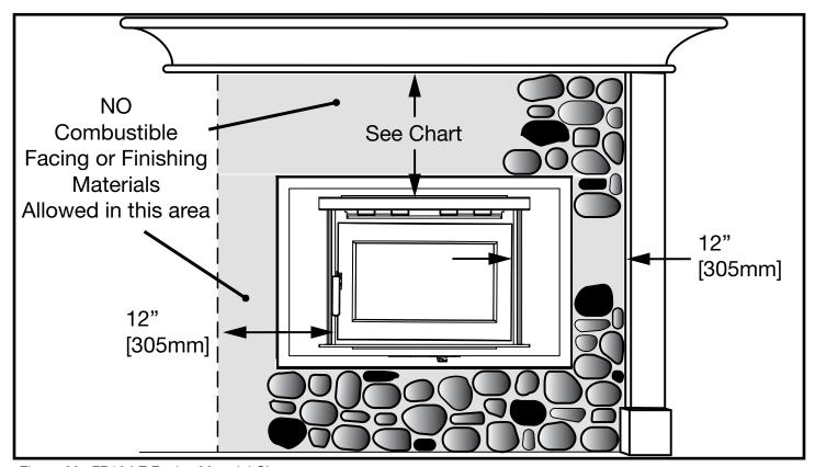
Figure 23: FP16 LE Facing Material Clearances.
