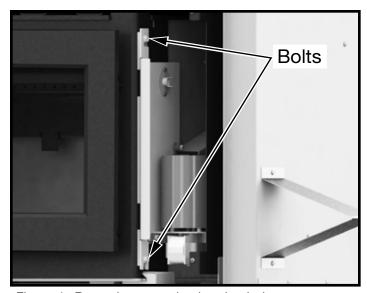
Figure 4: Removing mounting bracket bolts.
