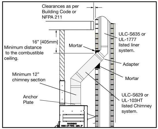
Figure 13: FP16 LE Masonry Installation.
