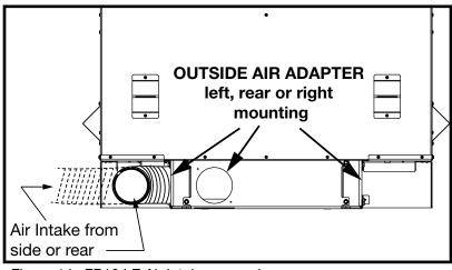
Figure 14: FP16 LE Air intake - rear view.
