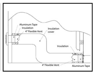
Figure 15: FP Typical outside air installation.
