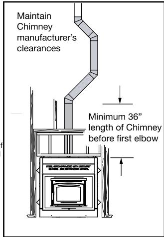
Figure 12: FP16 LE Offset Installation.
