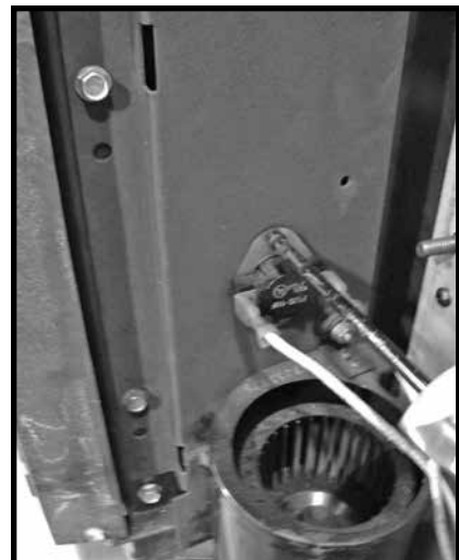
Figure 22: Unscrew thermal snap switch.
