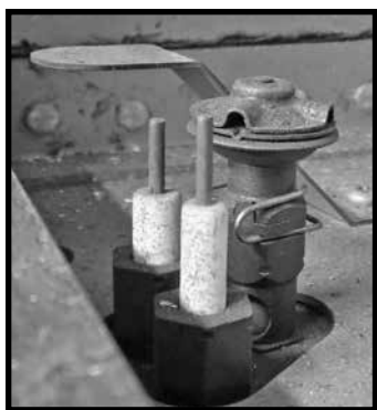
Figure 70: Trenton pilot assembly.
